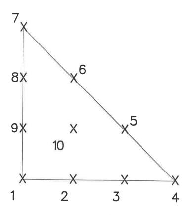
Figure 4: Local element numbering for the 10-noded cubic triangle.
