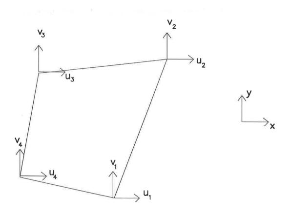
Figure 1: Velocity components on the bilinear quadrilateral element.
