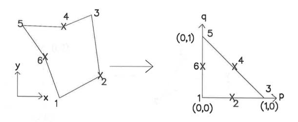
Figure 3: Transformation of the general quadratic triangle onto the standard element.
