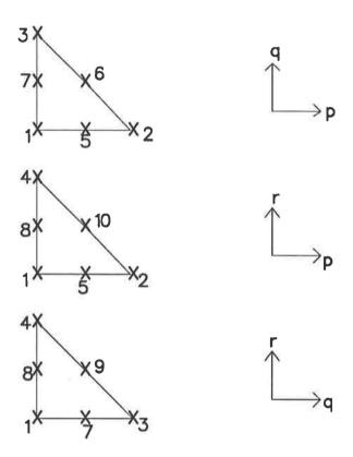
Figure 5: Local element numbering for the 10-noded tetrahedron.
