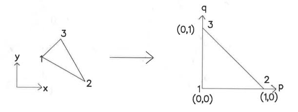
Figure 2: Transformation of a general triangle onto the standard element.
